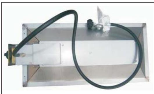
1. Make 2-3 oz. of leak check solution (one part liquid dishwashing detergent and three parts water).
