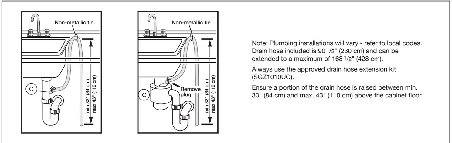
Note: Plumbing installations will vary - refer to local codes. Drain hose included is 90 1/2" (230 cm) and can be extended to a maximum of 168 1/2" (428 cm).
