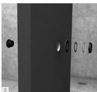
**GB** Set up a continuous 1/4" bead of wedi sealant along the top side of the wedi One Step valve groove profile. Drop the drain body firmly into the sealant. Turn the One Step pan upside down and apply the rubber and the fiber gasket. Tighten the gaskets firmly to the pans steel ring.
