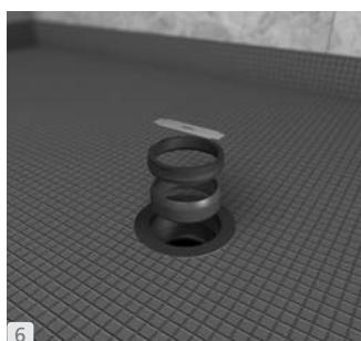
**GB** Set up the rubber caulking gasket (bevelled side up) around the 2" pipe in the subfloor. The rubber gasket must be flush with the upper end of the 2" ABS or PVC pipe. Tighten the connection using caulking nut, metal guide and screw driver.
