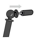
Hang the completed assembly by loosening the brackets front adjustment screws and dropping the rods in. Once hung, tighten both the brackets tighening screws and the connector tightening screws.
