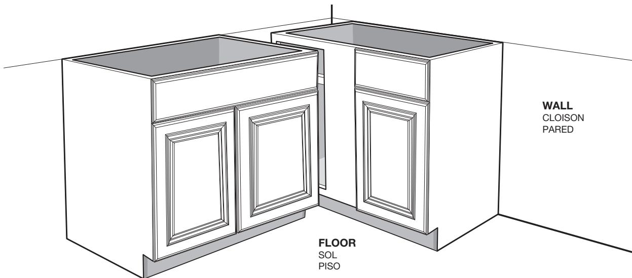
**5** Install a base filler to give proper door and drawer clearance between the blind base and adjacent cabinet. Clamp the filler to the face frame. Mark the location of the filler on the inside of the frame. Drill two (2) 1/8" pilot holes through the face frame and into the filler. Use two (2) #8 x 2" cabinet screws to secure the filler.
