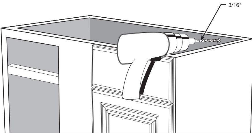
**4** Place the adjacent cabinet into place according to your design layout. Make sure the cabinets are level and straight.
