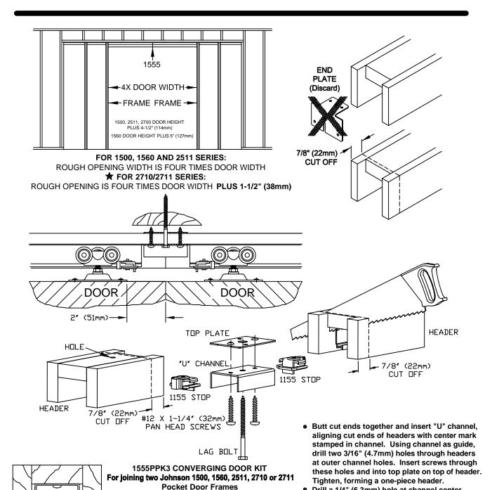
Remove and discard end plates from "door opening" end of each header.
