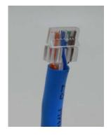
5) Place liner over trimmed conductors. Wire tips should touch closed end of liner.
