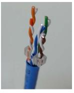
3) Place sled over twisted pairs. Place pairs based on 568A or 568B order.
