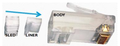
Liner "fin" points in same direction as plug pins. Here, the pin is down, and the fin is down. This shows the correct order and orientation of the 3 pieces to seat the wires correctly.
