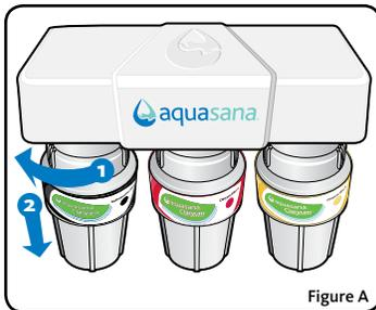
3. Remove each cartridge sump from the filtration system by rotating the sump towards the left side & pull down to detach. (Fig. A)
