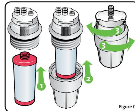
5. Insert & connect the new filter cartridge to the top half of the sump then reattach the bottom of the sump to the top half by turning & tightening clockwise. (Fig. C)
