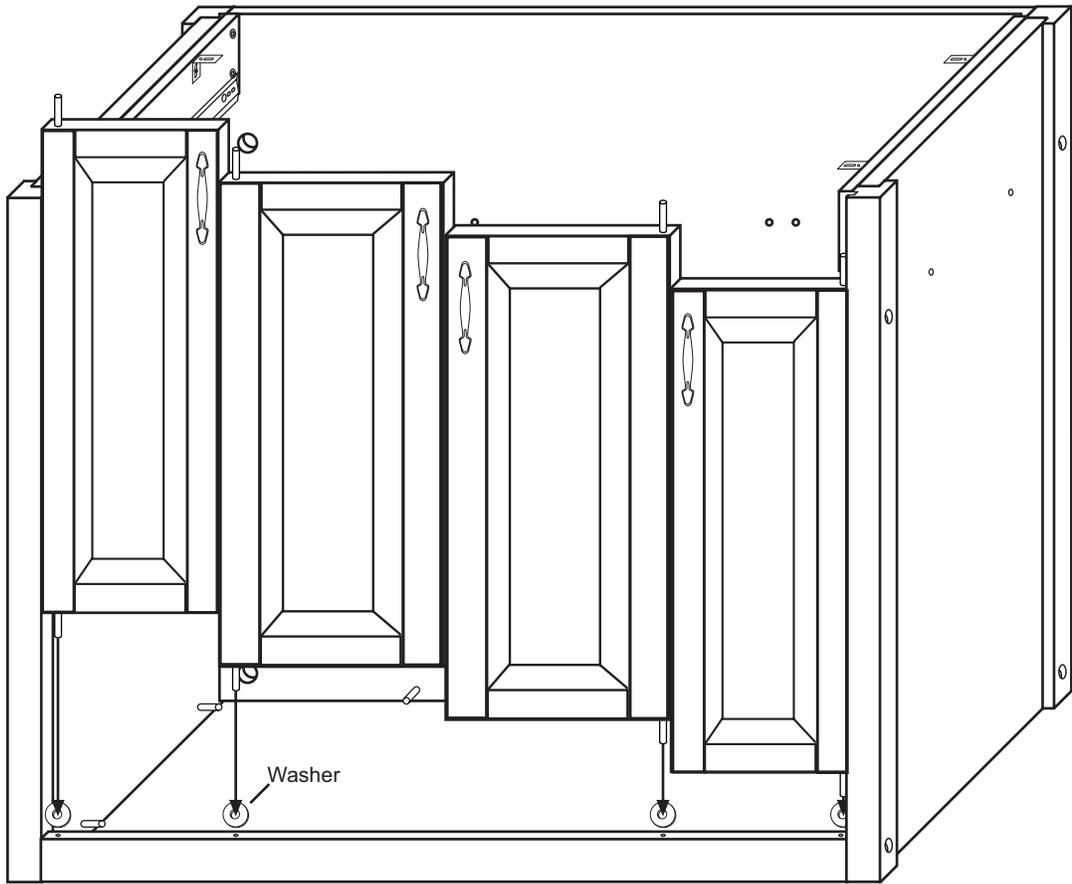
Slide top front brace down into position to secure doors. Fasten with 1 3/4" bolts and nuts as shown.
