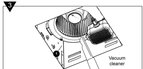
4. Dampen cloth with dust detergent and wipe the fan housing **1** . Then wipe dry with a clean cloth.
