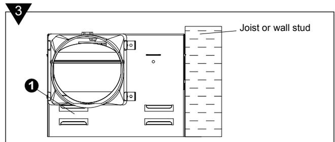
4. Mount the fan housing **1** to the joist or stud using nails (not included) where indicated.
