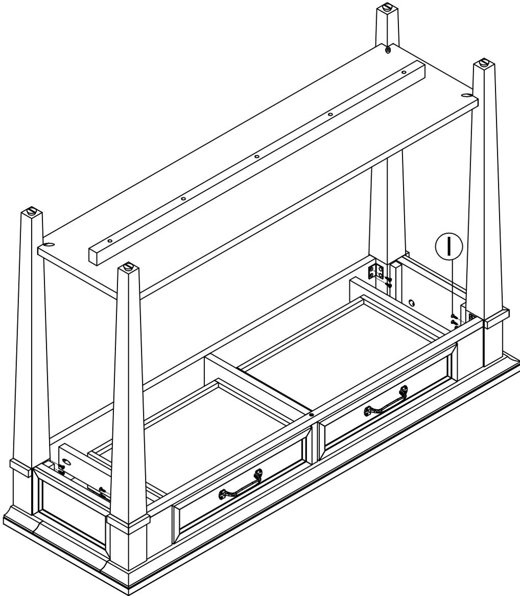
5). USE SCREWS (I) TO FIX L BRACKET (H) TO TOP PANEL (A) WITH SCREWDRIVER (NOT PROVIDED).
