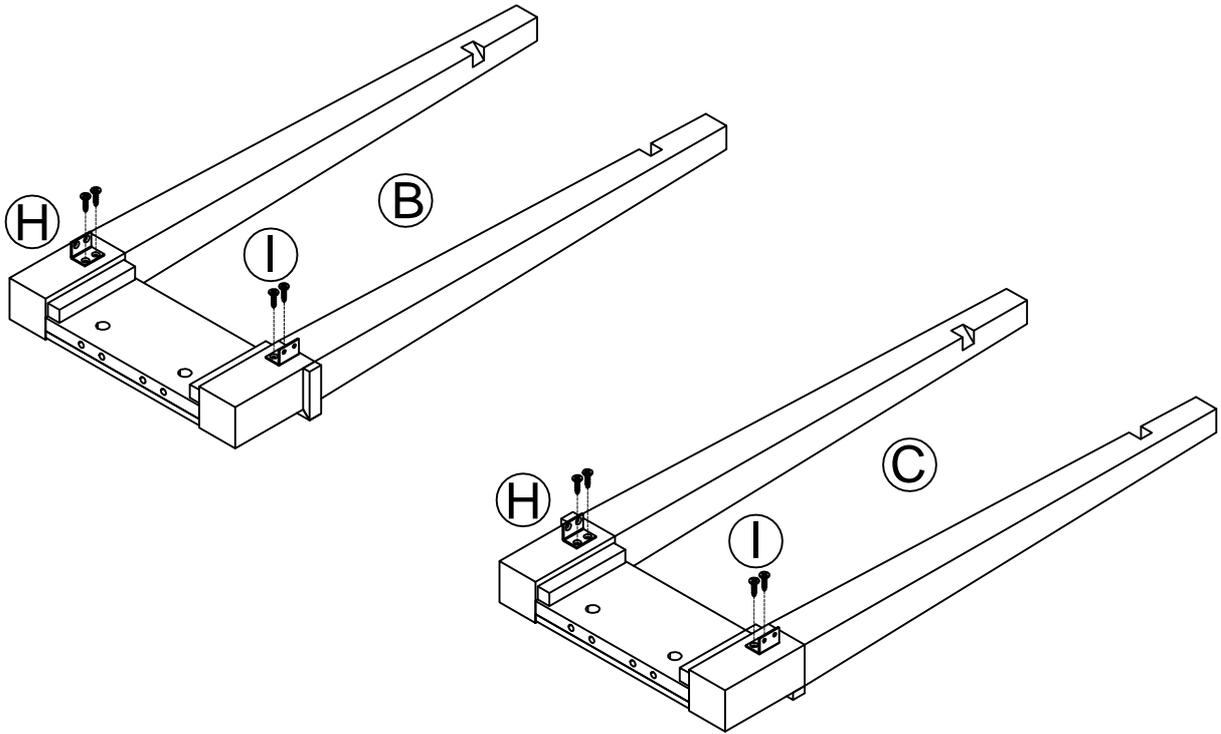
2) . USE SCREWS (I) TO ATTACH L BRACKET (H) TO LEFT SIDE FRAME (B) AND RIGHT SIDE FRAME (C) WITH SCREWDRIVER (NOT PROVIDED).
