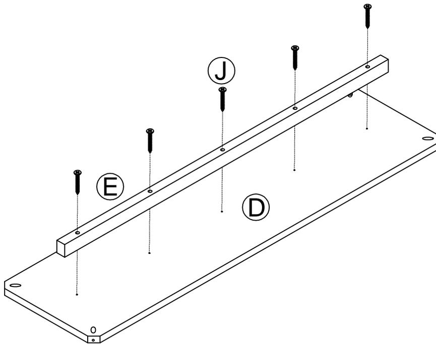
1). USE SCREWS (J) TO ATTACH SUPPORTING RAIL (E) TO SHELF (D) WITH SCREWDRIVER (NOT PROVIDED).
