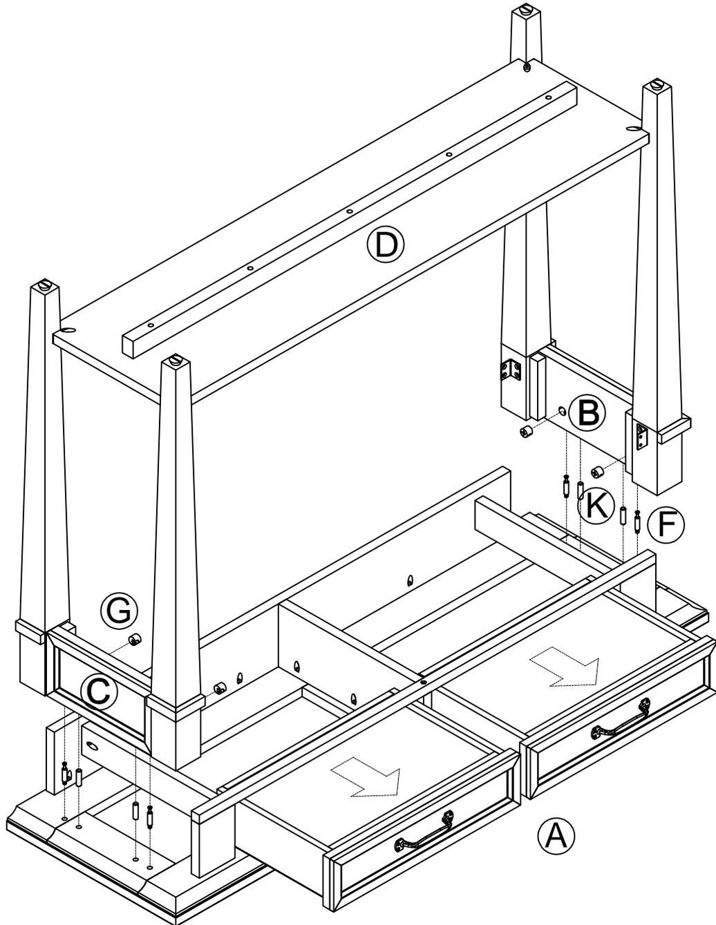
4). POSITION LEFT SIDE FRAME (B) AND RIGHT SIDE FRAME (C) TO TOP PANEL (A) BY USING WOOD DOWELS (K), CAM BOLTS (F) AND CAM LOCKS (G) WITH SCREWDRIVER (NOT PROVIDED).
