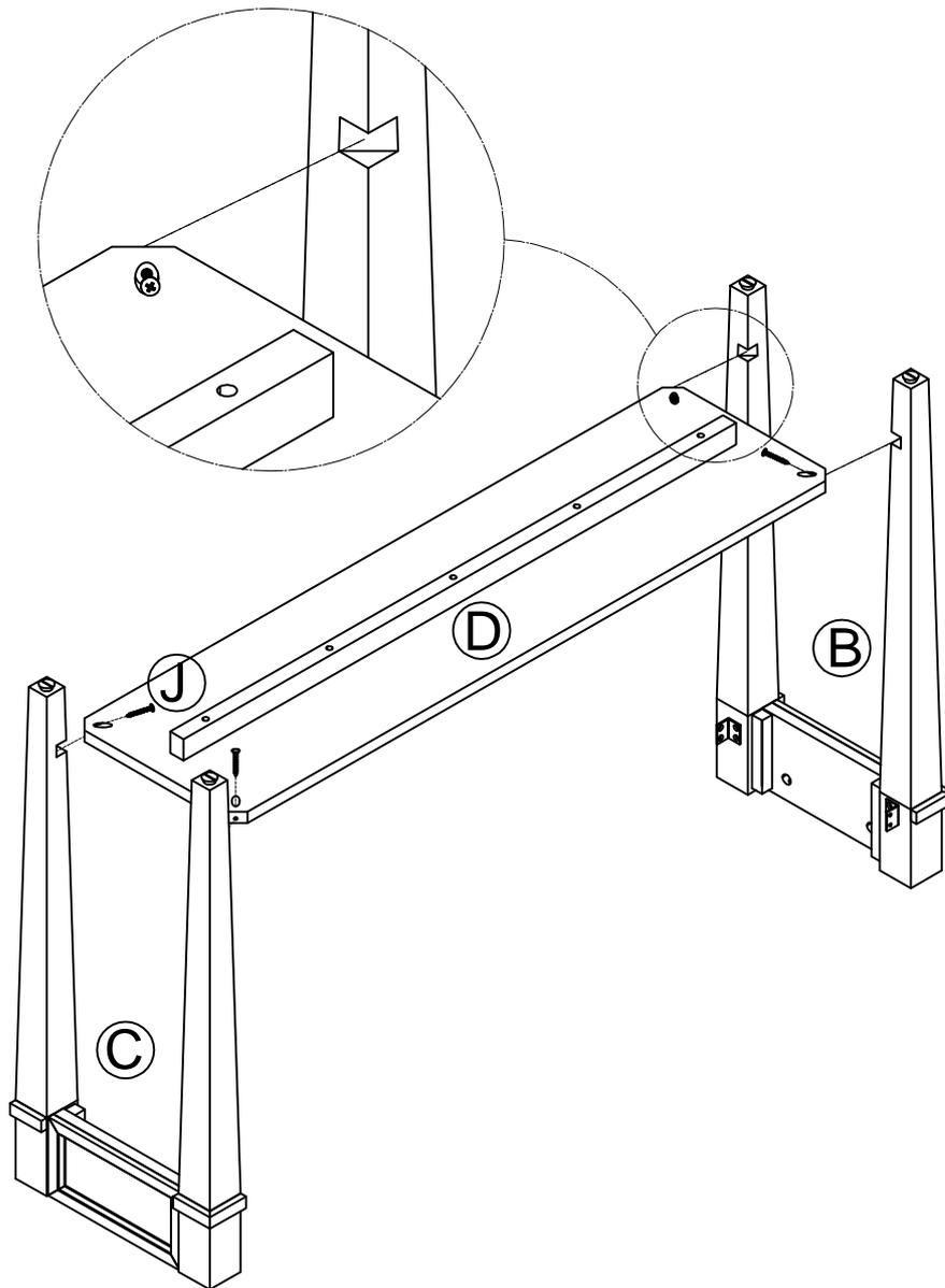
3). USE SCREWS (J) TO CONNECT SHELF (D) WITH LEFT SIDE FRAMES (B) AND RIGHT SIDE FRAMES (C) WITH SCREWDRIVER (NOT PROVIDED).
