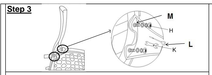
Attach the Studs(M)(M8\*30mm) to the contact points on Chair Seat Panel (B)using the Screwdriver (L).
