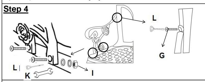
Connect the Right arm(E) and Left arm (F) to the Seat Panel (B) using Bolts, Washers, Spring washers and Nuts (6mm)(I).
