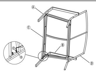
Attach Left Armrest/Leg(B) to Backrest(D) and Seat(C) using Bolts(②) and Washers(④) with Allen Key(①).
