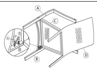
Attach Left Armrest/Leg(B) to Backrest(D) and Seat(C) using Bolts(2) and Washers(4) with Allen Key(1).
