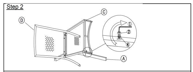
Place the Right Armrest/Leg(A) onto a clean, non-marring surface. Attach the Right Armrest/Leg(A) to Backrest(D) and Seat(C) using Bolts(②) and Washers(④) with Allen Key(①).
