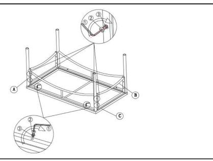
Attach the remaining Leg(A) to the Table Top(C) and Support Panels(B) using Bolts(②) and Washers(③) with Allen Key(①).
