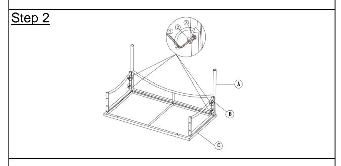
Attach Support Panels(B) to Table Leg(A) using Bolts(②) and Washers(③) with Allen Key(①).
