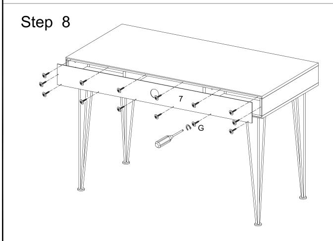
Attach the back panel (7) to the desk and secure it with screw (G).
