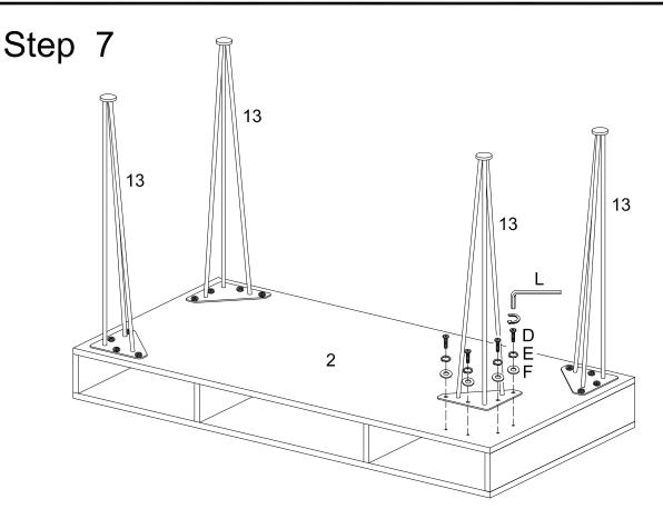
Attached the chrome legs (13) to the bottom panel (2) and secure it with washer (D), spring washer (E), bolts (D) and wrench (L).
