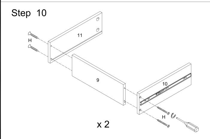
Assemble the drawer side panel (10,11) to the drawer back panel (9) with screw (H).
