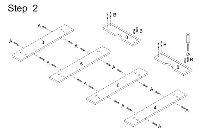
Insert the wooden dowel (A) to the side panel (3,4,5,6). Insert the cam bolts (B) to the drawer front panel (8).
