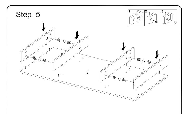
Assemble the side panel (3,4,5,6) to the bottom panel (2) and secure it with cam locks (C).
