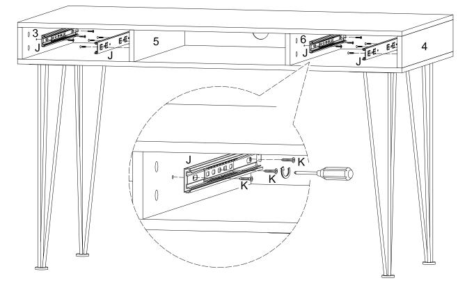
Assemble the drawer tray arms (J) to the side panel (3,4,5,6) and secure it with screw (J).
