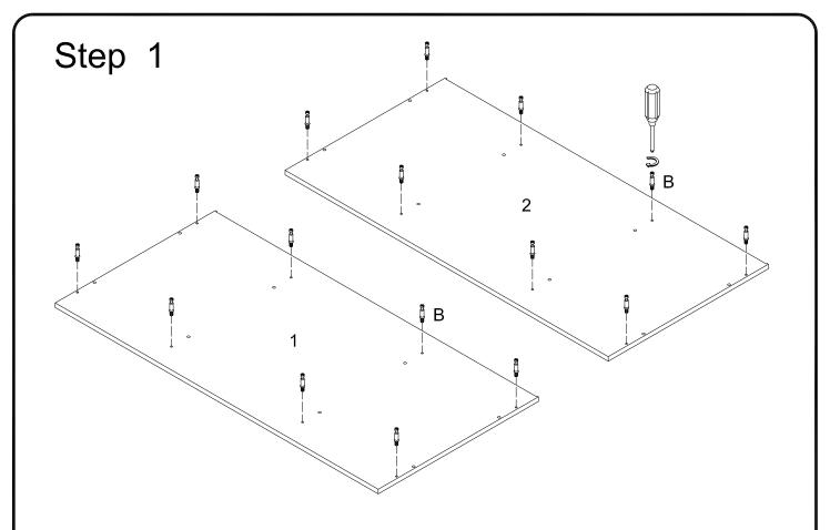
Insert the cam bolts (B) to the top (1) and bottom panel (2).
