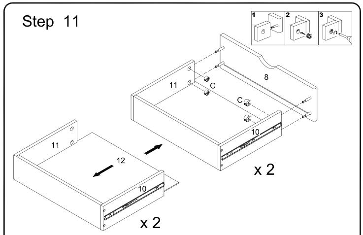
Slot in the drawer bottom panel (12) to drawer side panel (10,11) and use cam locks (C) to secure the drawer front panel (8) to the drawer side panel (10,11).
