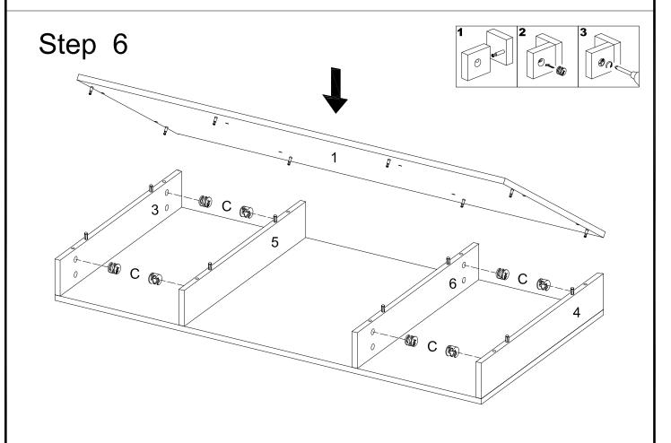
Place the top panel (1) on top of the side panels (3,4,5,6) and secure it with cam locks (C).
