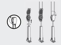
2. CEILING INSTALLATION. If rod is to be installed to ceiling, attach pulley housings (without brackets) and stirrup portion of center support directly to ceiling.
