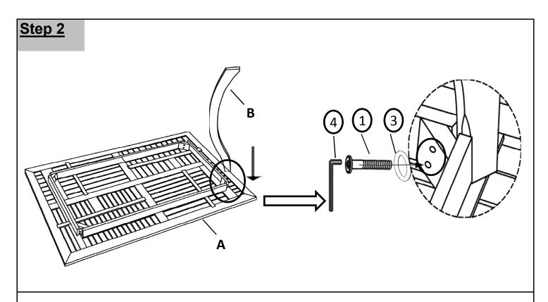
Attach Leg(B) to the Table Top(A) using Bolt(1) and Washer(3) with Allen Key(4).
