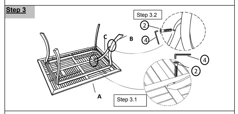
Place Leg Support(C) between Table Top(A) and Leg(B), as shown above.
