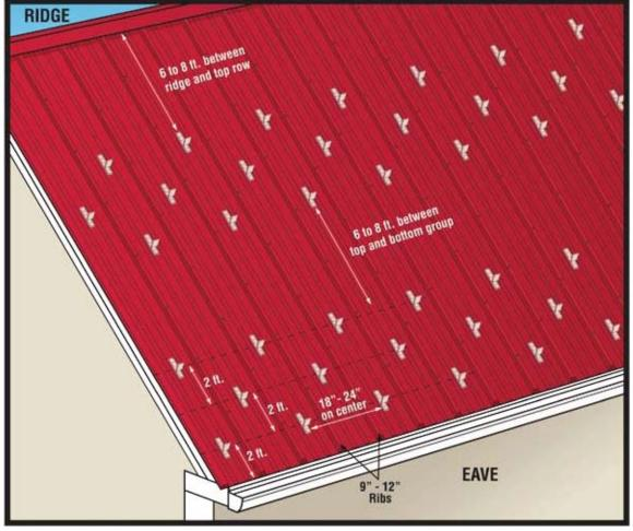
Horizontal spacing will be dictated but how far apart the metal seams or ribs. Shown is a typical RTMINI application on a 9" or 12" center rib panel. Do not place Snow Guards beyond the bearing wall on an extended roof section. Please see Appendix page A7 for general installation information.
