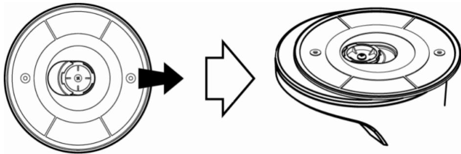
**2** Making sure that the
