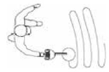
• It is better you sweep the search coil from side to side in an arc line of 3 inches motion and keep the search coil parallel with the ground.
