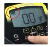
a. Press NOTCH and then press + or - to select the Target Indicator to be notched. The cursor above the selected target will flash.
