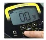
Press NOTCH again and the selected target ID will disappear. It means that this target will be notched during the detection, and the detector will have no reaction to the notched target.
