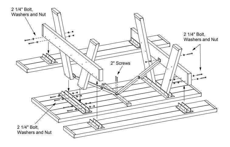
Insert one cross brace / leg assembly into brackets on underside of table top with cross brace closest to table end. Using four 2¼" bolts, washers and nuts, fasten assembly to table top. Repeat with second cross brace / leg assembly for opposite end of table.
