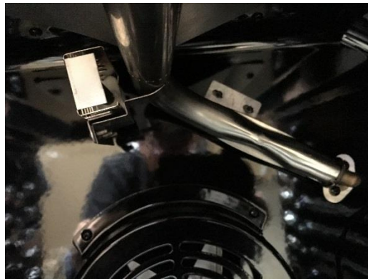
a. Broiler Burner is connected to Flame Tamer; b. Two screws on the back holding the burner to back oven panel;
