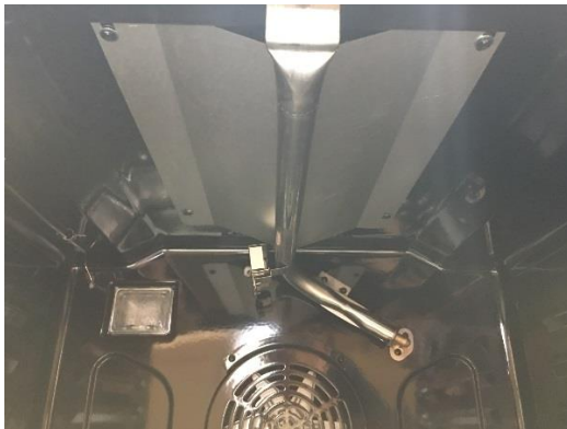
a. Broiler Burner is connected to Flame Tamer; b. Two screws on the back holding the burner to back oven panel;
