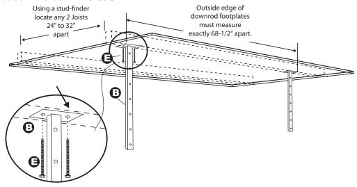
**1A:** Place Downrod (B) against ceiling under joist location and mark holes running parallel with the joist. Pre-drill each hole location using a 3/16" drill bit. Rub bar soap or add a drop of liquid soap to the threads of the Lag Screws (E) to ease installation. Install Downrod (B) using 1/2" Socket Wrench or Nut Driver and (2) 5/16" x 2-1/2" Lag Screws (E).
