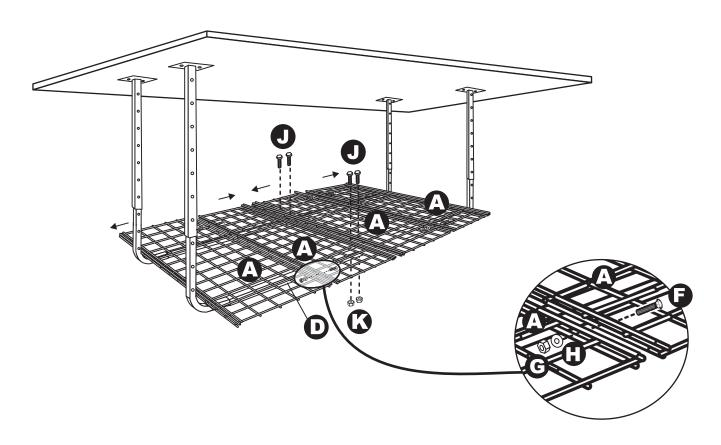
**3A:** Place Grids (A) across the two hanging Support Bar (D) assemblies making sure the long wires of the Grids (A) are facing down and the overhang is even on both sides.
