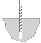
2. Drill 3/8" diameter holes 3" deep into surface. Make sure the holes are at least 3" away from any cracks in the base material.
