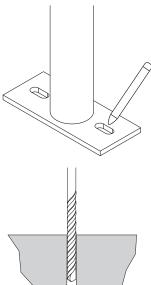
1. Place the rack in the desired location. Use a marker or pencil to outline the holes of the flange onto the base material.
