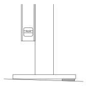
3. Place rack (and washers to level rack if necessary) over holes.
