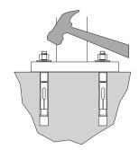
4. Thread nuts onto anchors, leaving approximately 1/4" of the anchor protruding, and tap into surface. Tighten nuts down to secure rack.
