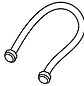
Toilet water supply line
