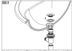
As shown. Insert Flange with Washer through Sink drain Hole. From underside, thread Drain Body into Flange. Holding the drain body in position with Ball Rod Opening facing back, tighten Metal Locknut securely. Thread Drain Tailpiece into Drain body.
