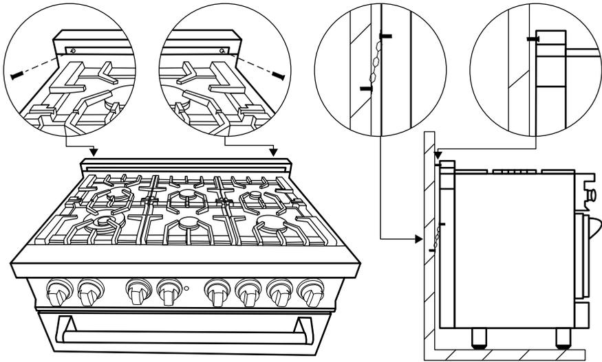
1. Measure the distance from the floor to the where the chain connects on the back of the appliance.
