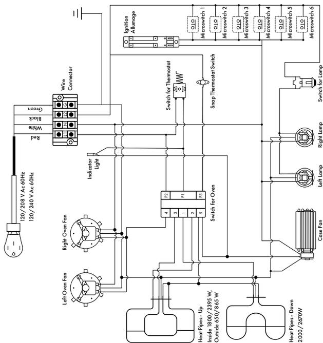
**CAUTION:** Connect the red wire to the L1 tab (left), the black wire to the L2 tab (right), the white wire to the N tab (central), and the yellow and green wire to the ground screw. DO NOT SWAP CONNECTIONS.
