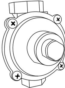
The pressure regulator shipped with the appliance has two female threads 3/4" NPT. The regulator shall be installed properly in order to be accessible when the appliance is installed in its final position.
