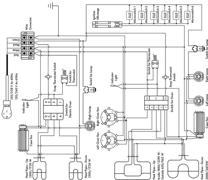
**CAUTION:** Connect the red wire to the L1 tab (left), the black wire to the L2 tab (right), the white wire to the N tab (central), and the yellow and green wire to the ground screw. DO NOT SWAP CONNECTIONS.
