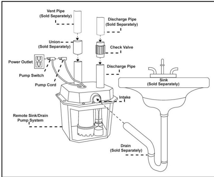
3. Connect the vent pipe of the remote sink/drain pump system to the vent pipe (sold separately) using a union (sold separately).
