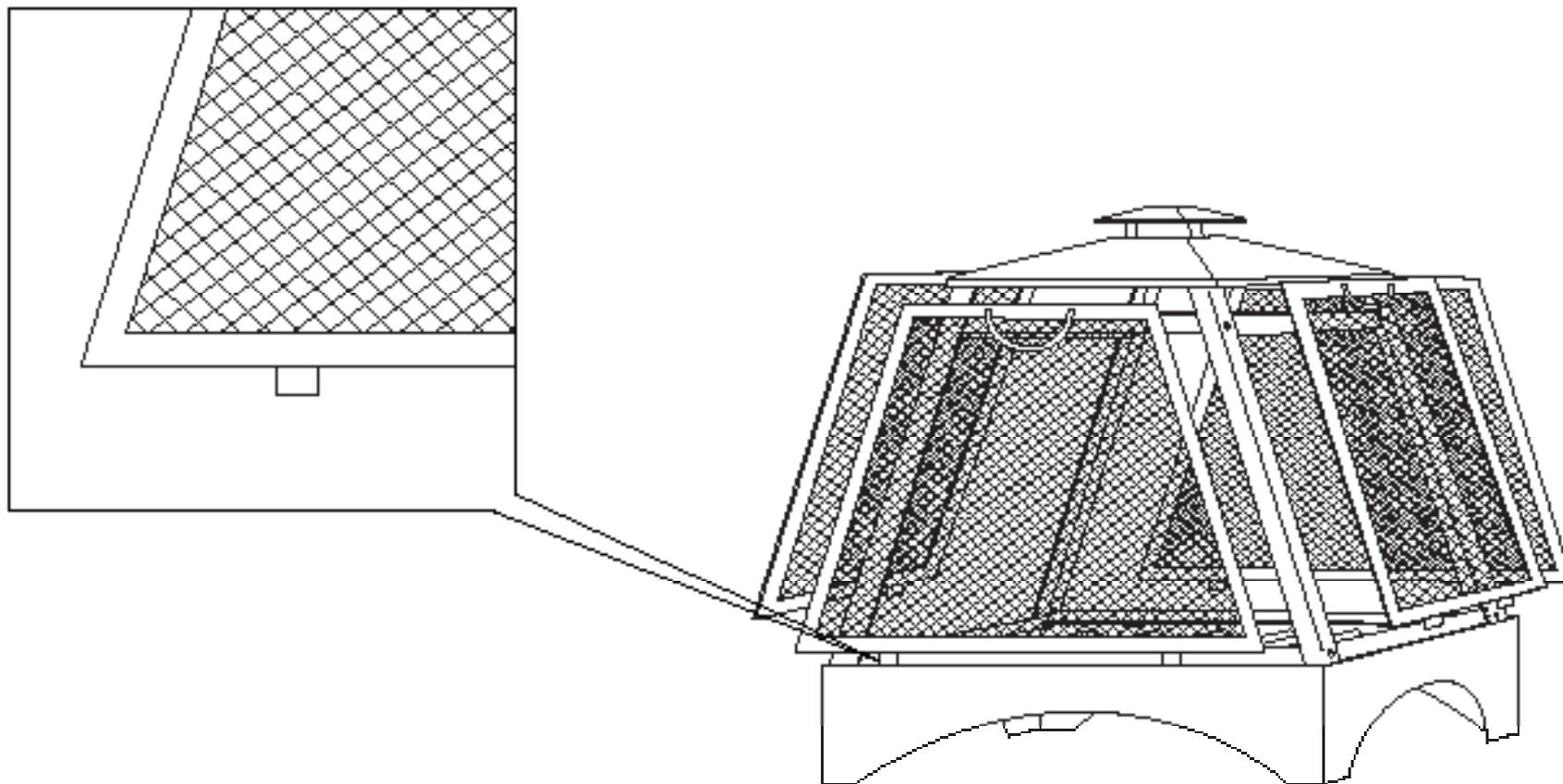
1. Place Screens (E) on each side of frame, inserting screen tabs into base tab notches.
