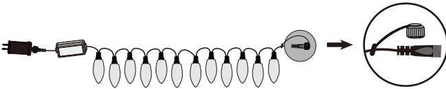
6. Connect the two kits together. Tighten the lock nut to secure the connection.
