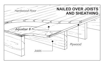
coverage. Overlap edge seams a minimum of 4 inches. Once **Aquabar "B"** is installed, snap chalk lines to desired layout.
