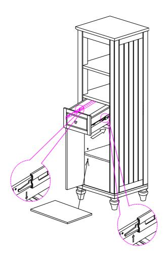
Pull the right clip upward and left clip downward at the same time, then draw the drawer box out.
