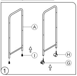
Step 1: Insert End Cap (I) into Side Frame (A).
