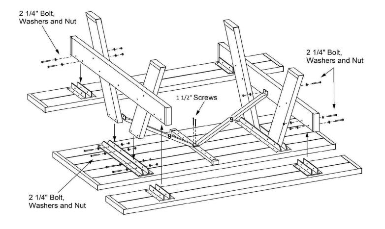
Insert one cross brace / leg assembly into brackets on underside of table top with cross brace closest to table end. Using four 2¼" bolts, washers and nuts, fasten assembly to table top. Repeat with second cross brace / leg assembly for opposite end of table.
