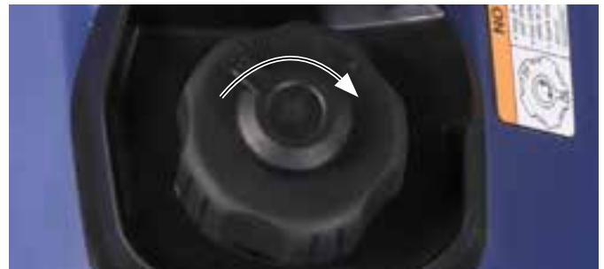
Figure 7: Turn Fuel Vent to ON
