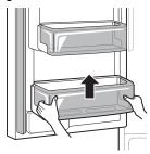
To assemble the bin, slide it in above the desired support and push down until it snaps into place.
