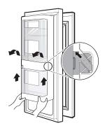
Pull out the crisper to full extension, lift the front up, and pull straight out.
