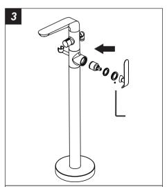
Place a new cartridge in the cartridge seat, then screw the cartridge lock nut and assemble the handle by securing the screws. Repeat the above steps for the other cartridge if necessary.
