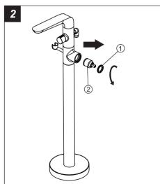
Unscrew the cartridge nut① with adjustable wrench, then take out the old cartridge②.
