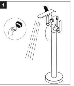
Remove aerator by coin and open the hot and cold water supplies. Check for leaks. Turn on faucet handle for one minute to flush debris from faucet.
