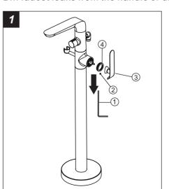
Disassemble the screw② with allenkey①, take out the handle③, then remove the trim cap④.
