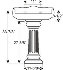
Dimensions of fixture are nominal and may vary within the range of tolerances established by ASME Standard A112.19.2-2008. Dimensions and specifications subject to change without notice.
