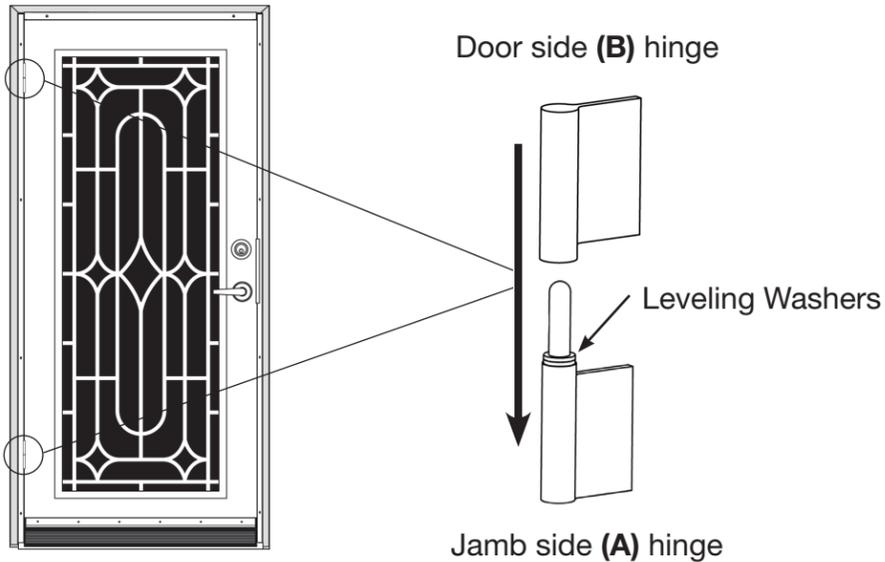
Hang the security door (B) on the jamb hinges (A), holding the door open at more than a 90° angle (see diagram below), starting with the bottom pin first.
