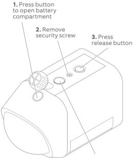
**4.** Remove weather seal, and insert in unused hole
