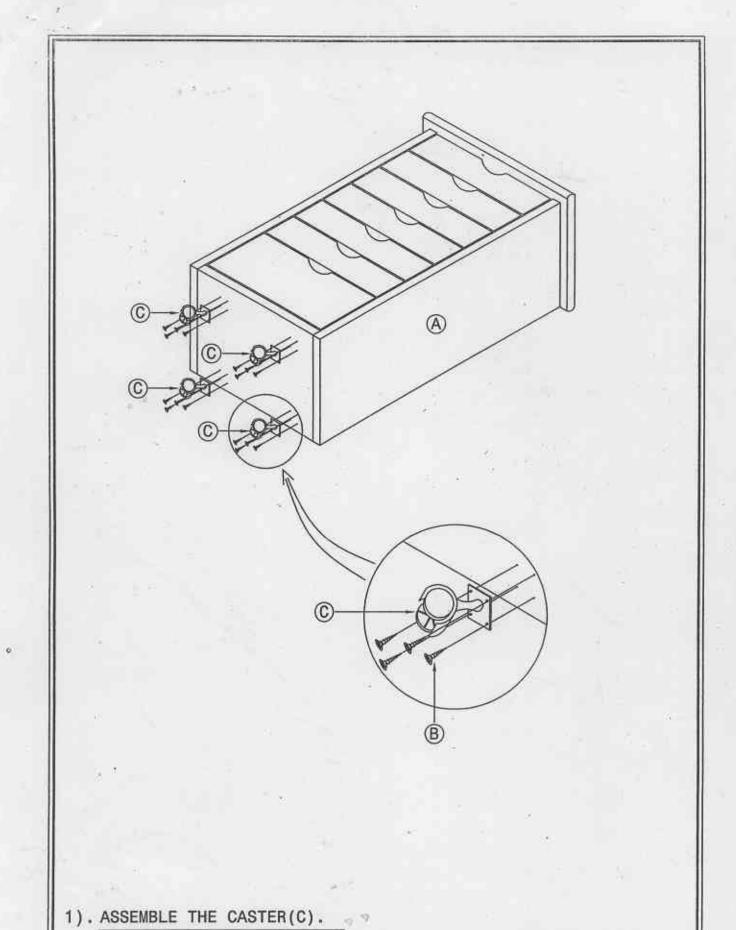
. ATTACH CASTER(C)TO BOTTOM PANEL OF CABINET(A)USING 16 SCREWS(B).
