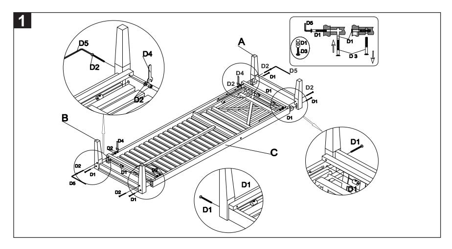
Step1: attach the rear leg (A) to the seat (C) as shown on the picture by using the Allen bolt (D1) and Allen nut (D2). Tighten all with the Allen key (D4) and Wrench (D5). Repeat the assembling of the front leg (B) in the same way as the rear leg (A). Tighten all bolts and screws again before use.
