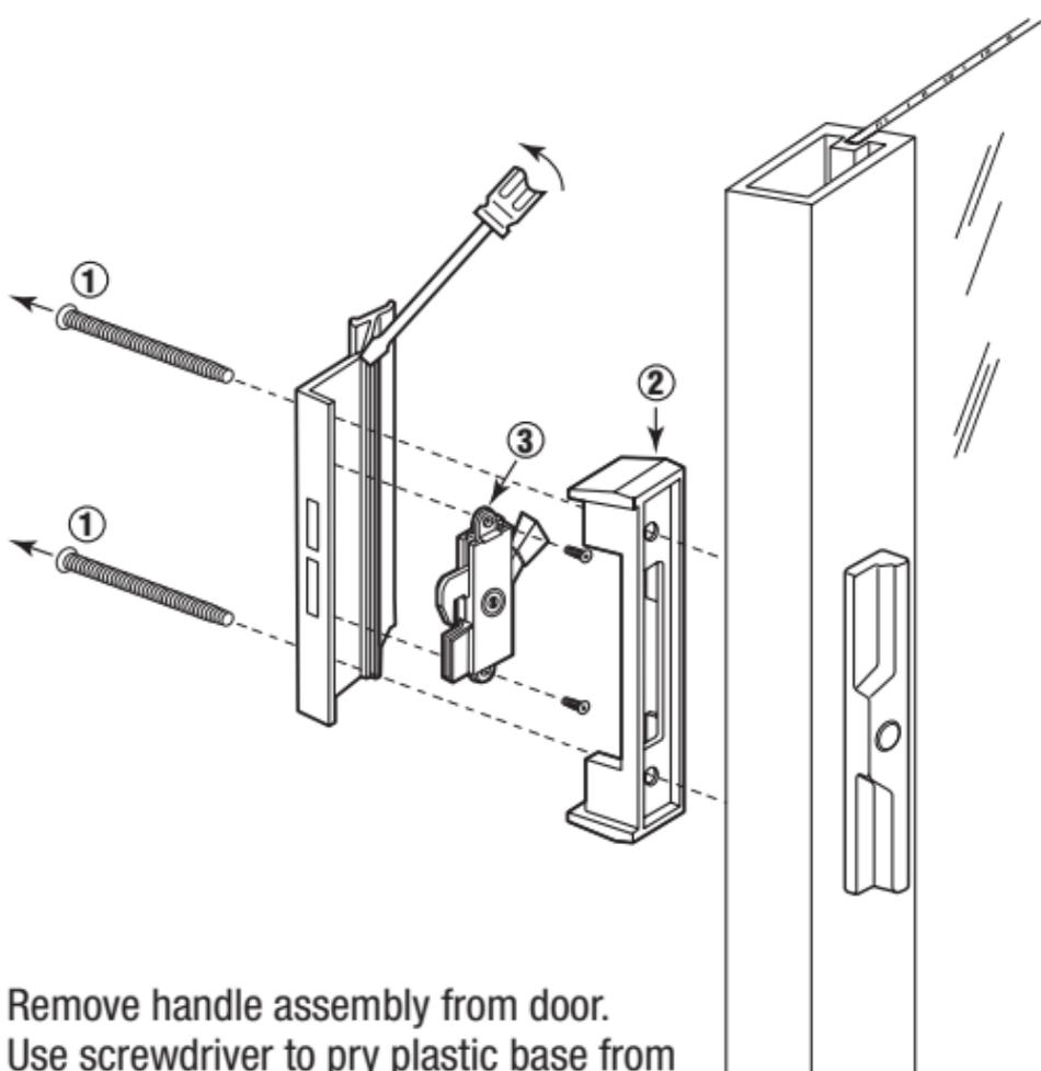
Remove handle assembly from door. Use screwdriver to pry plastic base from aluminum handle. Base should snap-off easily. Replace existing latch with hook in same position. Replace plastic base and re-mount handle.
