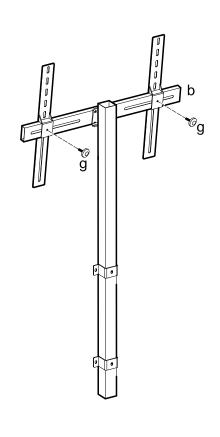
Slide mounting bars (c) onto lateral support bar (b). Secure mounting bars (c) by screwing adjustment knobs (g) into place.
