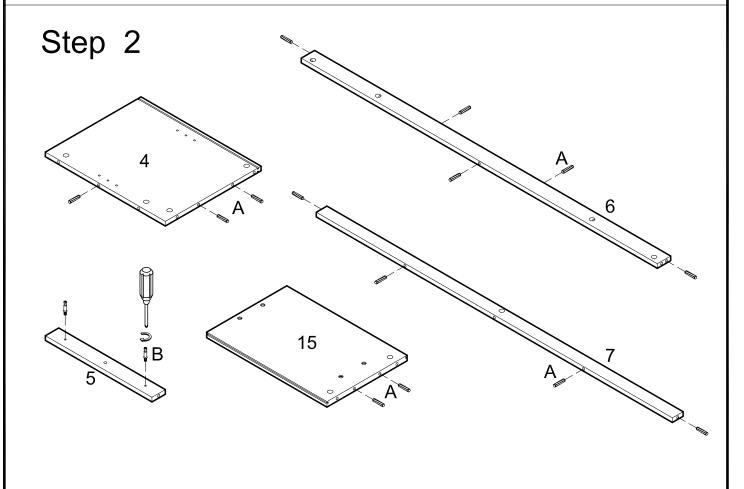
Insert dowels (A) into panel (4,15) and slats (6,7). Screw cam bolts (B) into slat (5).
