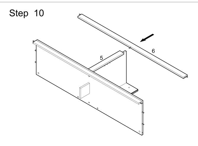
Attach slat (6) to slat (5) using dowel as guide.
