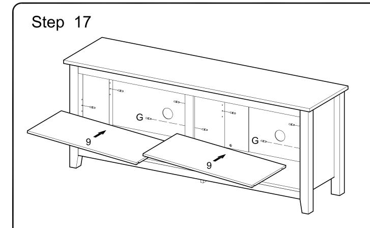
Insert shelf support pins (G) into the assembly at desired shelf heights. Carefully place shelves (9) on shelf support pins (G).
