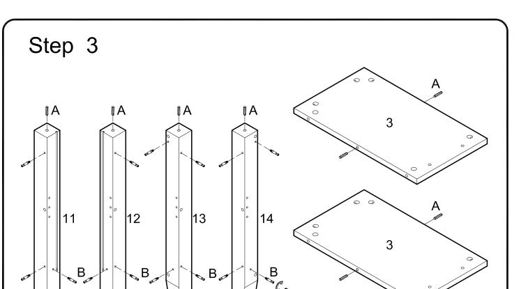
Insert dowels (A) into legs (11,12,13,14) and panels (3). Screw cam bolts (B) into legs (11,12,13,14).
