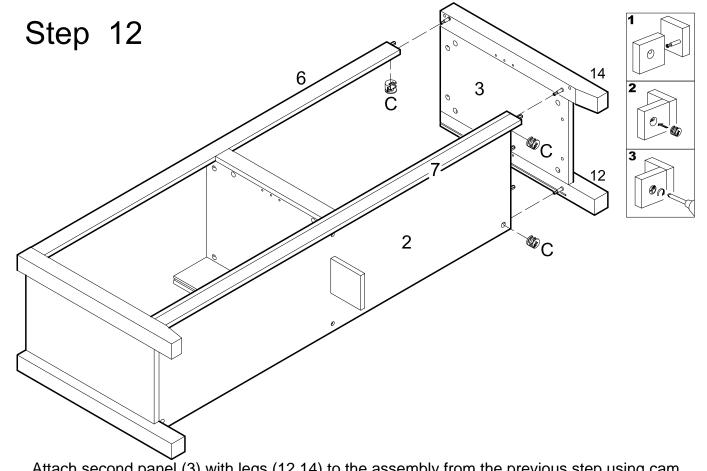
Attach second panel (3) with legs (12,14) to the assembly from the previous step using cam bolts and dowels as guides. Insert cam locks (C) into panel (2) and slat (6) and tighten with a screwdriver.
