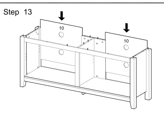
Carefully slide panels (10) into place along the back of the assembly.
