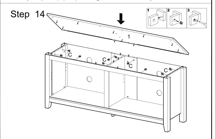
Carefully attach panel (1) to the assembly using cam bolts and dowels as guides. Insert cam locks (C) into the assembly as shown above and tighten with a screwdriver.
