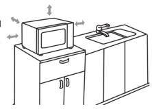
proper operation, the oven must have sufficient airflow. Allow 3 inches (7.6 cm) of space on both sides of the oven and 1 inch (2.5 cm) of space on top of the oven.
