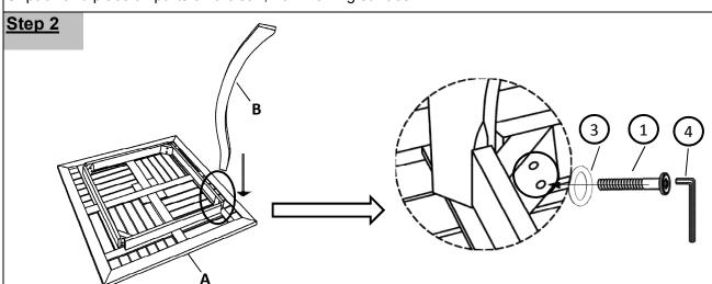
Attach Leg(B) to the Table Top(A) using Bolt (1) and Washer(3) with Allen Key(4).
