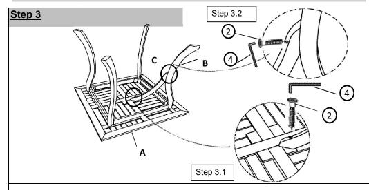
Place Leg Support(C) between Table Top(A) and Leg(B), as shown above
