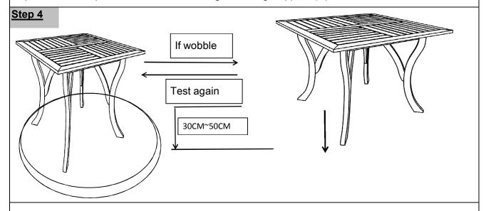
Place the Table right side up on a LEVEL SURFACE to see if it wobbles. If it wobbles, lift the Table to some 30cm to 50cm height from the ground. Keep your feet and toes well away from the drop zone.
