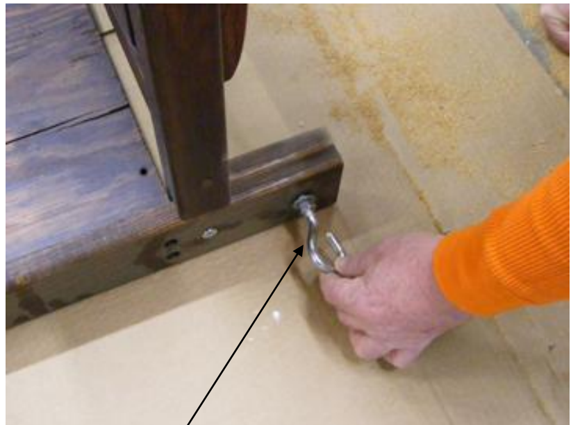
Fig.15 Opening shown up but install face down
