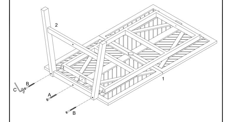
Using bolts (A,B) secure part (2) to part (1) with hex key (C) as per diagram.
