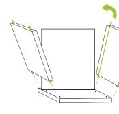
Carefully remove the 3M protective layer from adhesive.
