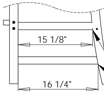
12° Compound angle cut with long edge on bottom
