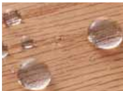
Water bead – the surface is not ready to coat and requires more preparation.
